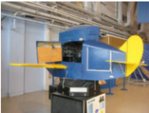
Figure 39 First simulator, image source: https://interestingengineering.com/transportation/the-worlds-first-commercially-built-flight-simulator-the-link-trainer-blue-box
