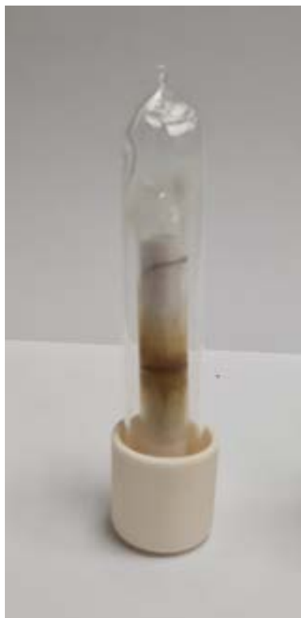
FIGURE 3.3: Photo of a double-sealed quartz tube, after heating. Dark marks can be seen on the contained crucible set.
