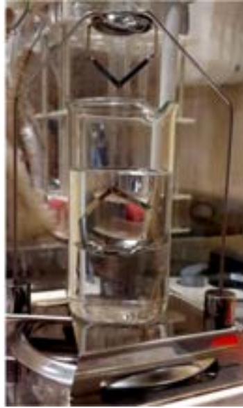
Figure 18. A balance prepared for Archimedes liquid displacement measurements.
