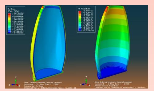
Equivalent stress in MPa calculated according to HMH criterion (left) and total deformation in m across the structure (right) for the load combination.
